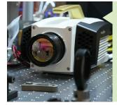
We are equipped with high resolution, high speed thermal cameras (up to 14 kHz frame rate) that can accurately evaluate the origin of unwanted thermooptical effects.
