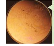
Presence of dust, organic contaminants, scratches and digs of an optical surface can be evaluated, preventing potential damages during high power laser operation.
