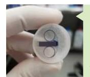
Careful optimization of the surface state, glue deposition method, and insulation time were conducted. and assessment of the process was verified with in-situ wavefront metrology and post-bonding glue thickness analysis.
