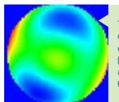
The transmitted wavefront error (TWE) of an optic can be evaluated on a large surface (up to 25 mm diameter), with a precision down to  $\lambda/20$  at 633 nm.
