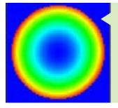
Optics with unknown radius of curvature can be accurately measured, whether convex or concave, from 2 to 50 m, for optics from 10 to 30 mm diameter.
